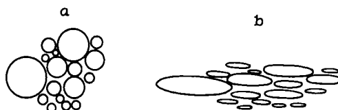
Fig. 3. Hypothetical change of pore shapes caused by stretching the membrane in one direction.
